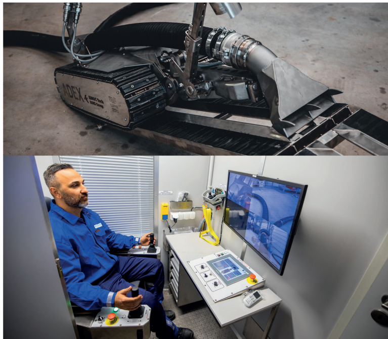
Operating the ATEX Zone 0 robot out of the transportable, vented cabin
