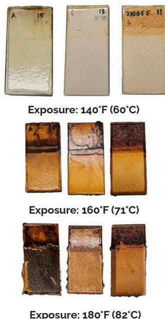
Figure 2. In cyclical testing (top), panels were immersed in vegetable oil and water at 180°F (82°C) for 30 days, then had 75% of the mixture replaced before the next cycle. A control set in continuous exposure with no cycling (bottom) showed much greater corrosion damage – even after shorter total exposure times.
